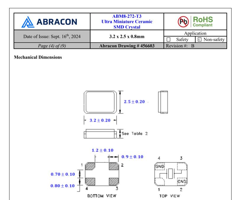
Note: Due to material availability, the chamfer could be located on pin #1, 3, or 4. Be advised that the chamfer location has no impact on the electrical performance of the device.
