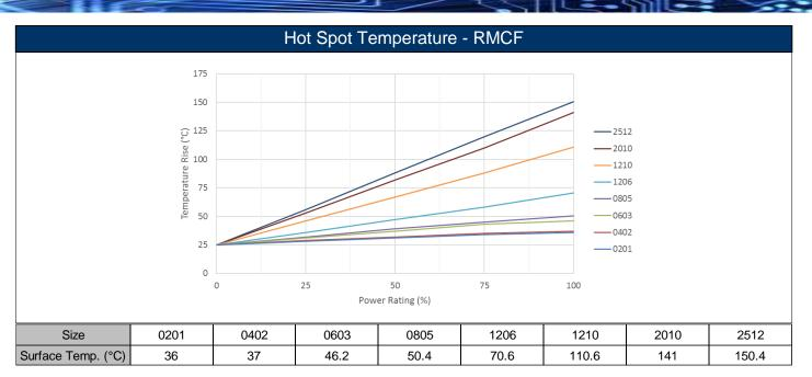
The thermal resistance of the RMCP will be similar to the RMCF. For example, the RMCF2512 and the RMCP2512 will have similar surface temperatures at 1W; the RMCP is designed to withstand higher temperatures associated with high power levels.
